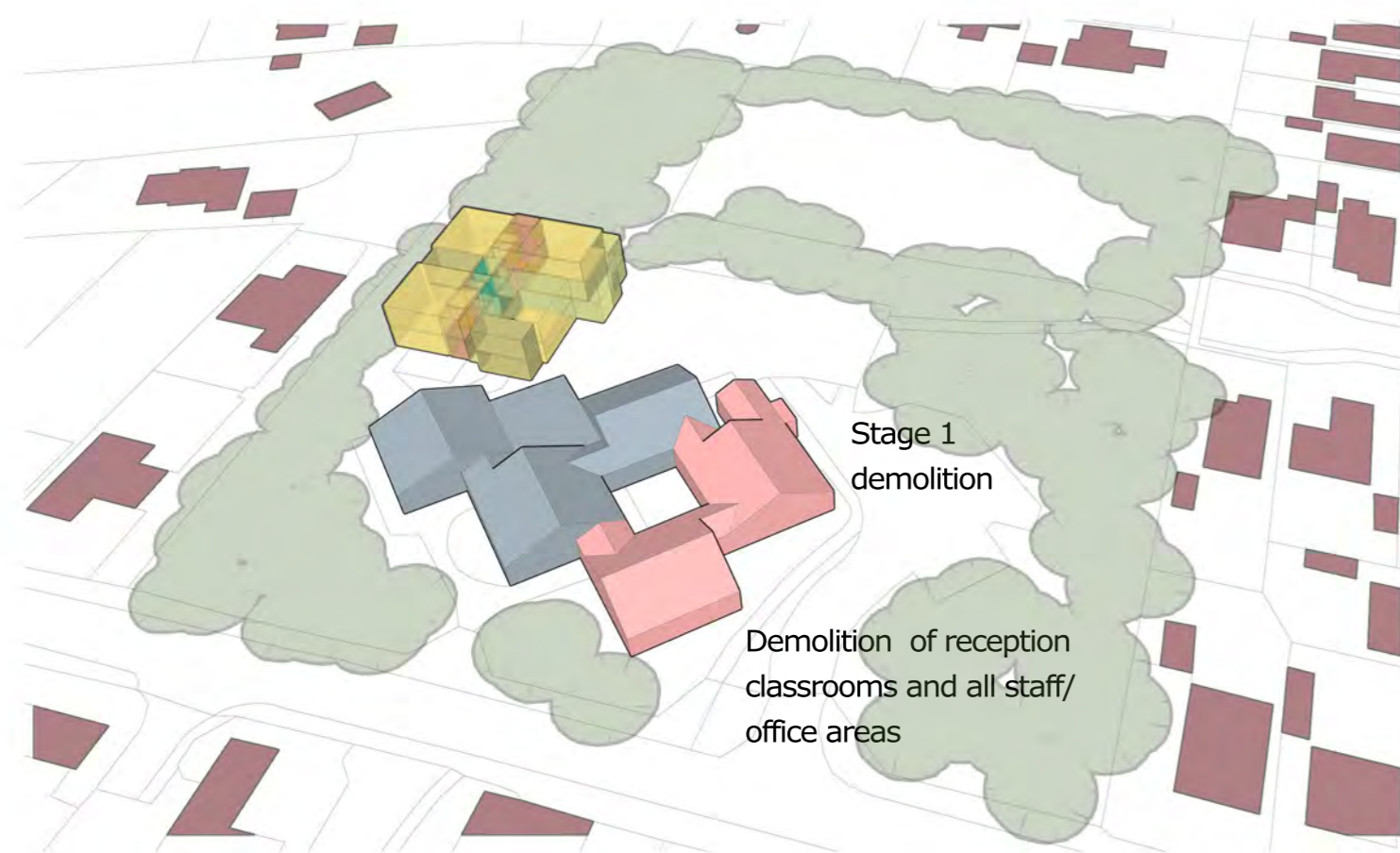
Phase 2 - 1st stage of Demolition.
